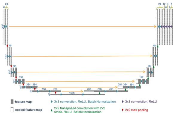
U-net architecture with additional CNN layers used for dose prediction. Source: Nguyen et al. (2019), picture courtesy of the authors.
